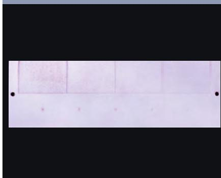
Type 3: JIMA PT TP-03 (AL burning crack specimen)
